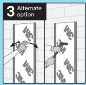
Wipe the membrane from the middle outward to obtain a smooth application, then roll with a rubber roller for a tight bond to the wall and overlaps.
